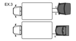
Distance A will be detected first, then distance B, as the car reverses. However, as the car nears, A will fall into the sensor's blind zone. In such cases, the system will misjudge B as the closest distance.
