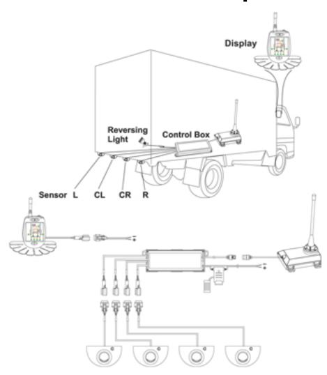
A. Conceal all cables starting at the display and beeper and work towards the control box. Use remaining cable ties to bundle any excess cable or wire. Be certain excess wire is secured and out of the way.
